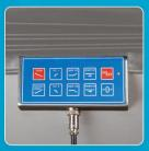
independent control panel with fail-safe system offers override function if remote control hand box in not availtable.
