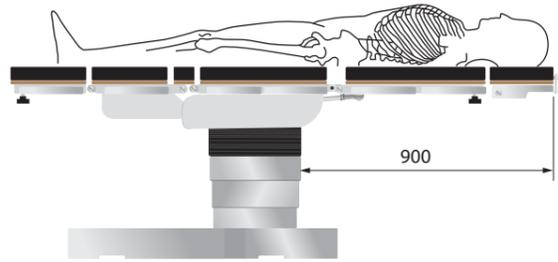
(Reverse Position / Head plate join in leg plate)
